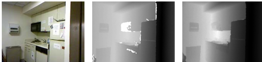
Fig. 2. Hole filling in depth images: 1) RGB image; 2) corresponding raw depth data; 3) depth data after applying the bilateral filter proposed in [13].
