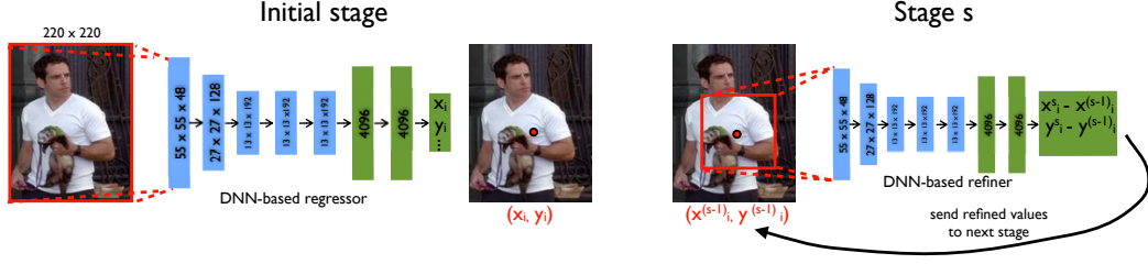
Figure 32 – Multi stage refinement of body pose estimation in DeepPose framework [297]. Convolutional layers are shown in blue and the fully connected layers are shown in green. The total number of stages in this implementation s \leq 3 .
